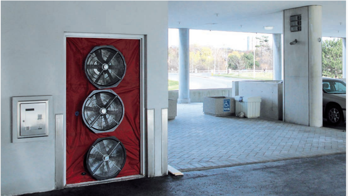
Typical blower door test at multi-story building
